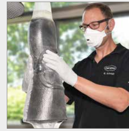
4. The titanium joint bars are laminated into the carbon construction.
