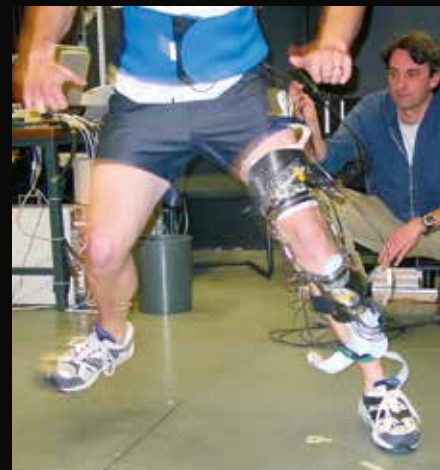
In the Vivo Workload Measurement of the subject groups at the German Sport University in Cologne so as to determine the stabilization characteristics of the K-COM knee brace.
