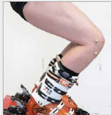
1. The 3D surface scan in different angular positions of the leg with set marker points forms the basis for calculating the frame design of the knee brace.
