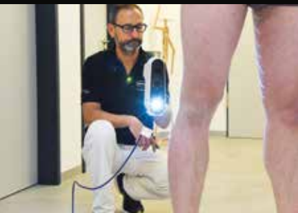
The 3D scan captures the circumferences and lengths of the leg extremely accurately.
